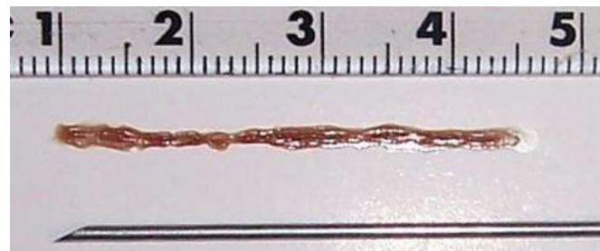
Needle tissue cutting tests to determine the sample length
