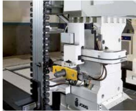
Chain-type tool magazine with 40/60 positions ISO50/HSK-A-100
