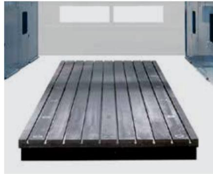
Cast iron worktable, independent from the machine structure, available in several sizes
