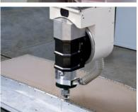
A suction system, developed by Jobs, equipped with programmable mobile hood can be integrated on these heads. This solution allows the maximum dust suction efficiency over the entire work area of the machine
