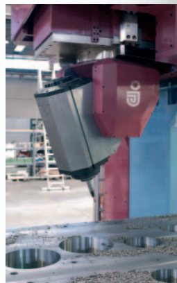
Universal bi-directional TMX head with electrospindle
