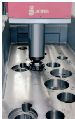
3-axis milling/boring head with external diameter 200 mm
