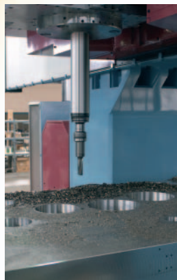
3-axis milling/boring head with external diameter 100 mm
