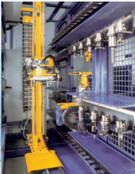
Modular rack-type tool magazine (HSK-A-100) with large storage capacity, pre-arranged for twist and angular heads.
