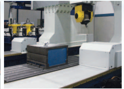
X and Y axis protections with roller coverings (pedestrianised for X axis).
